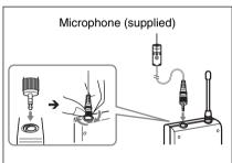
For a secure connection, be sure to turn and lock the connector cover.
